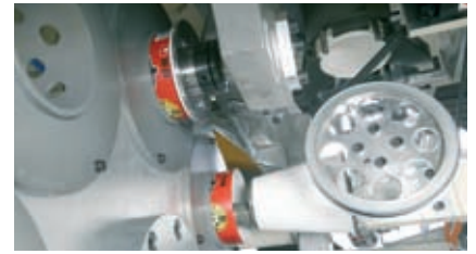
Insertion of the cup into the pre-glued outer shell
