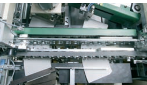
Gluing and heating of the blank
