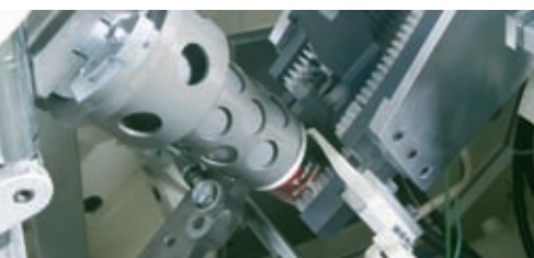
Tight and accurate wrapping by means of brushes and folding fingers.
