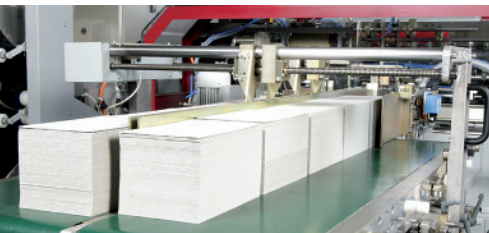
Board pre-pile belt
