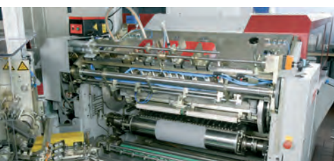
Short gripper cylinder transfer path ensures precise register
